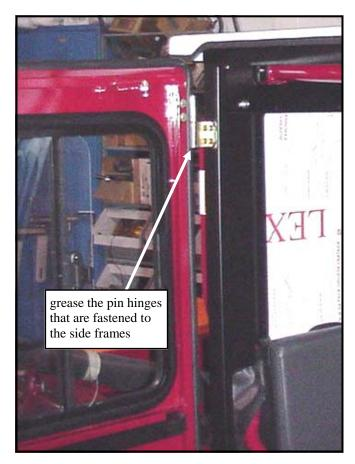
Fig. 13.1 (view from passenger's side) (hard sided door shown)
